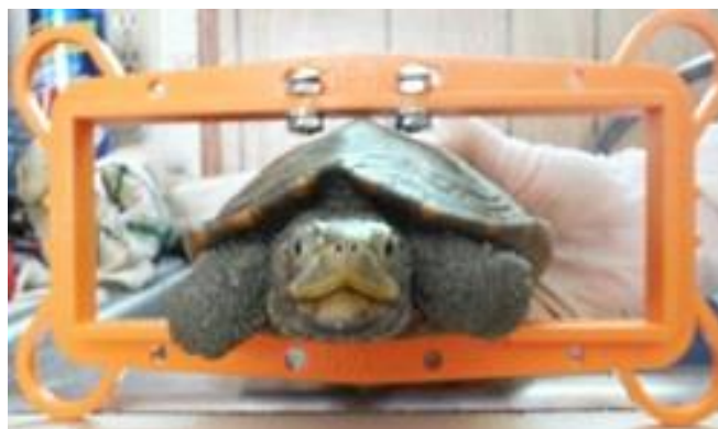
An example of a plastic terrapin excluder device (Source: South Carolina Department of Natural Resources)
